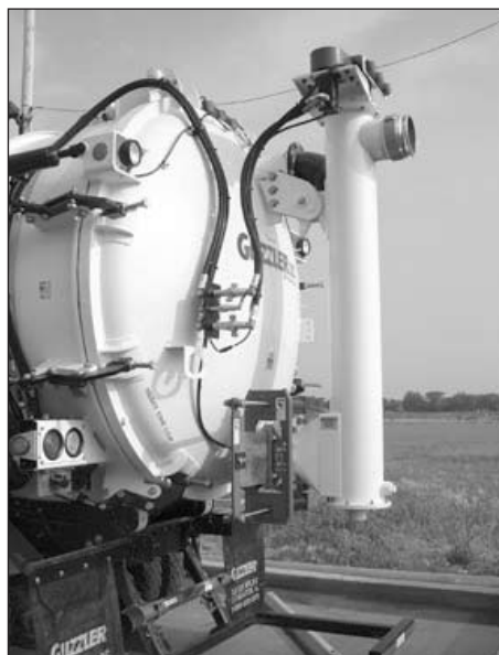
Guzzler's vertical auger system.
