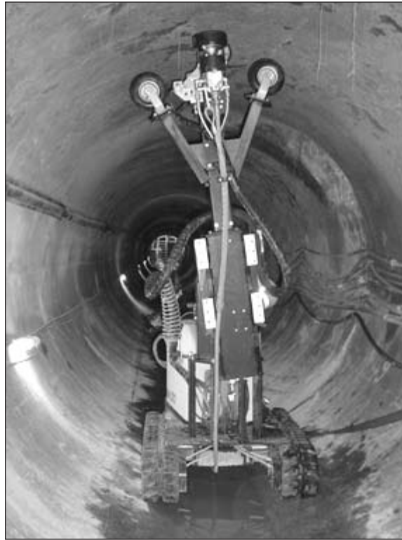
The compact Conjet Robot 322, here fitted with a rotor head, is ideal for working in small tunnels or similar structures with restricted access.
