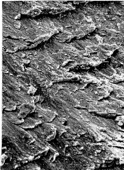
Figure 7. Traces of seizing on the workpiece surface of PA1 alloy machined with a grinding wheel with loaded working surface (x100).
