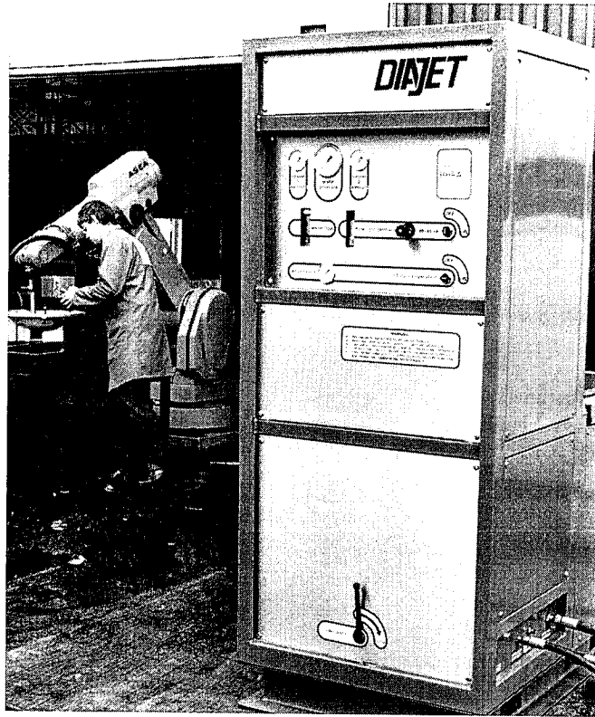
Fig 7 DIAJET site module used for trials of robot automated fettling of castings
