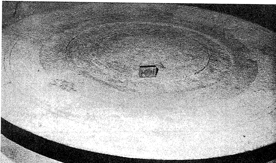
Fig. 13. One of the samples after mining process with a disk cutter and the assistance of high-pressure water jets.
