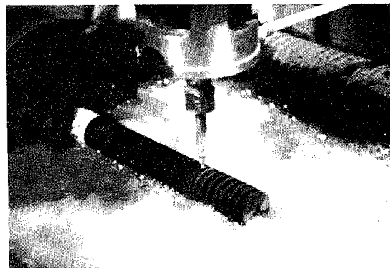
b. Helical shape machined by an AWJ traveling over the centerline of a rotary part
