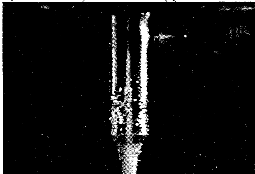
c) Lch = 25 mm, Lab= 10.72 mm, P=300MPa, (Qair max. = 65 l/ min; Pv = 93 mbar)
