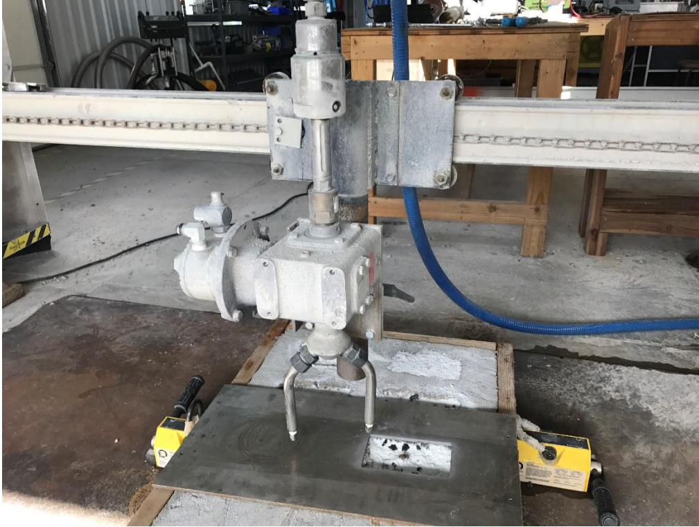
Test Arrangement Consisting of Rotating Jet Head and Traverse Mechanism Figure 3.
